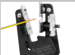
Automatic stripping of the insulation.
