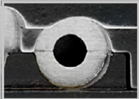
Stripping Area (Round Blades, no wire damage)
