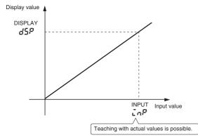
Instead of setting by inputting with the D Up Key and Shift Key, current values can be input as scaling input values for teaching. This is useful for making settings while checking the operation status of the K3MA-F.
