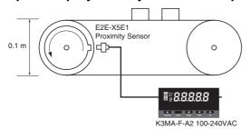
Here, the conveyor belt feed speed is to be displayed in units of 0.1  $\,\mathrm{m/min}.$
