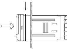
Fit the adaptor into the grooves on the left and right sides of the rear case, then push it until it contacts the panel to secure the K3MA-F
