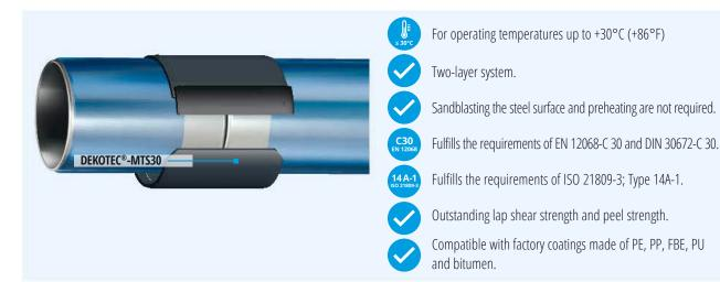
**DEKOTEC®-MTS30** is a heat shrinkable sleeve consisting of an electron beam cross-linked polyethylene carrier film and an adhesive on the basis of a polymer-modified bitumen for the corrosion prevention of the field joints at steel pipes.
